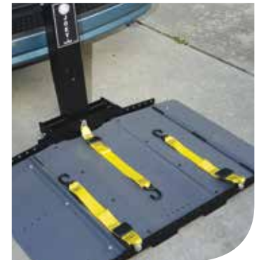
One-hand operation securement belts.
